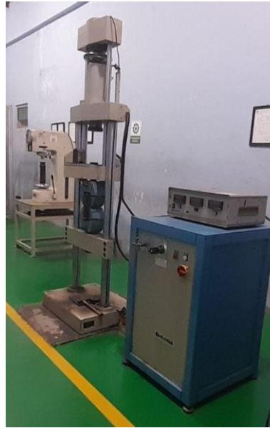
Gambar 5.15 Universal Hardness Tester, Universal Testing Machine (UTM), dan Impact Testing Machine
